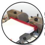
**Electric Double-Sided Crimpers** The adjustable knives provide consistent and perfect crimps, with a simple press of the foot pedal.
