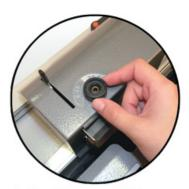
Adjust Crimper Knives on both sides according to your coil diameter size.
